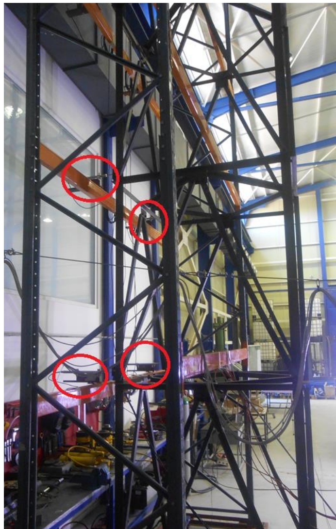
Figure 6.2: LVDTs measuring the horizontal displacements and supporting rack structure for orthogonal loading
