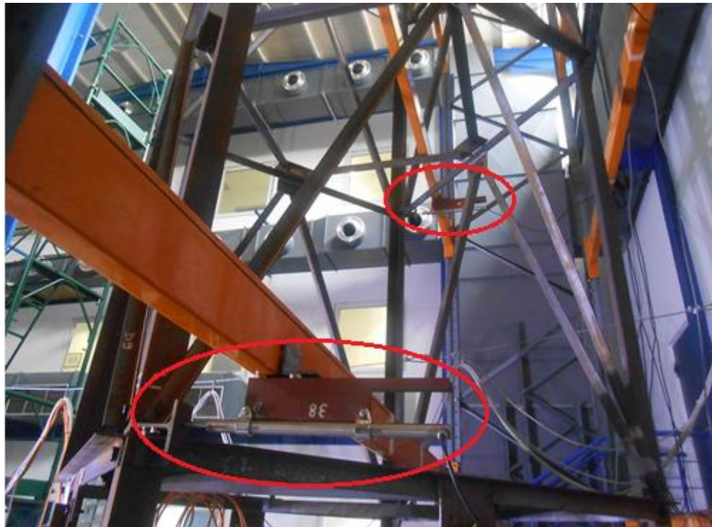
Figure 6.3: LVDTs measuring the horizontal displacements and supporting rack structure for diagonal loading
