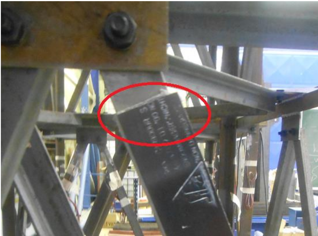
Figure 2.5: Outstand for wider FRP than angle leg L45.45.5
