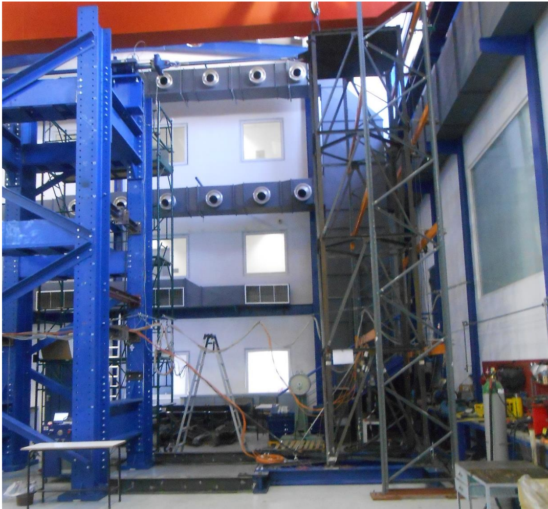
Figure 4.1: Reaction frame (left) and tower specimen (right)
